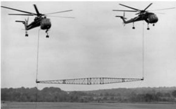
Figure 8: Army studies of twin-lift using spreader bars [Meek 1970]
