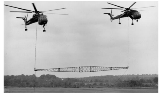
Figure 35: Ch-54B on a twin-lift mission
