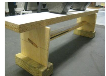
Figure 96: Jig built to impart nose-down twist to the baseline blades
