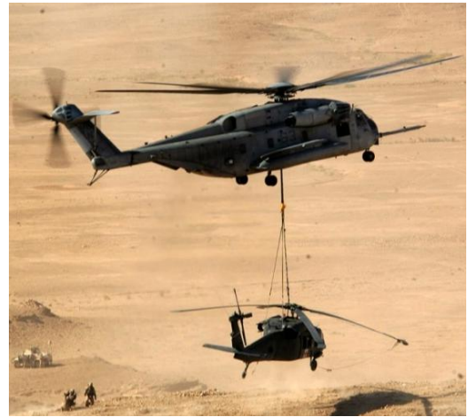
Figure 34: CH-53E carrying a UH-60 on a sling
