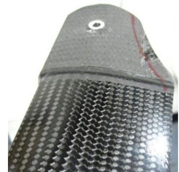
Figure 102: Blade root of optimized custom blades
