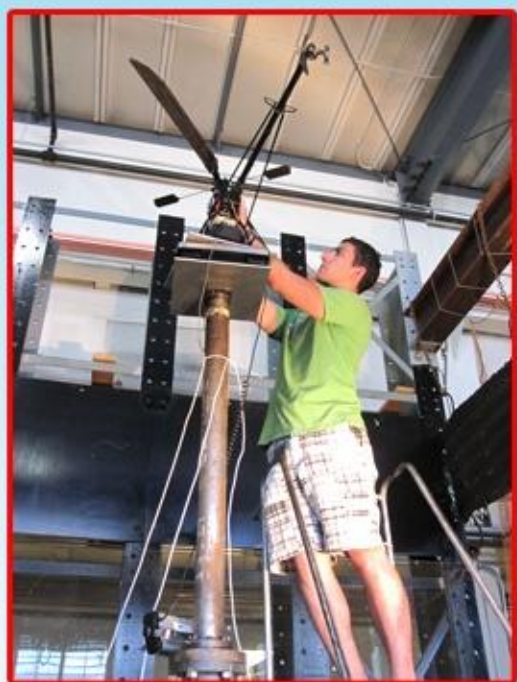
Mounting of Helicopter on UMD Alfred Gessow Rotorcraft Center Hover Stand
