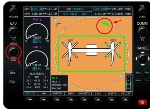
Figure 74: Avionics display for turn coordination
