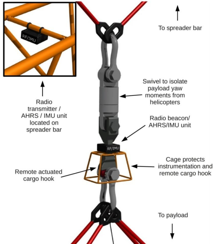
Figure 25: Remote-instrumented cargo hook
