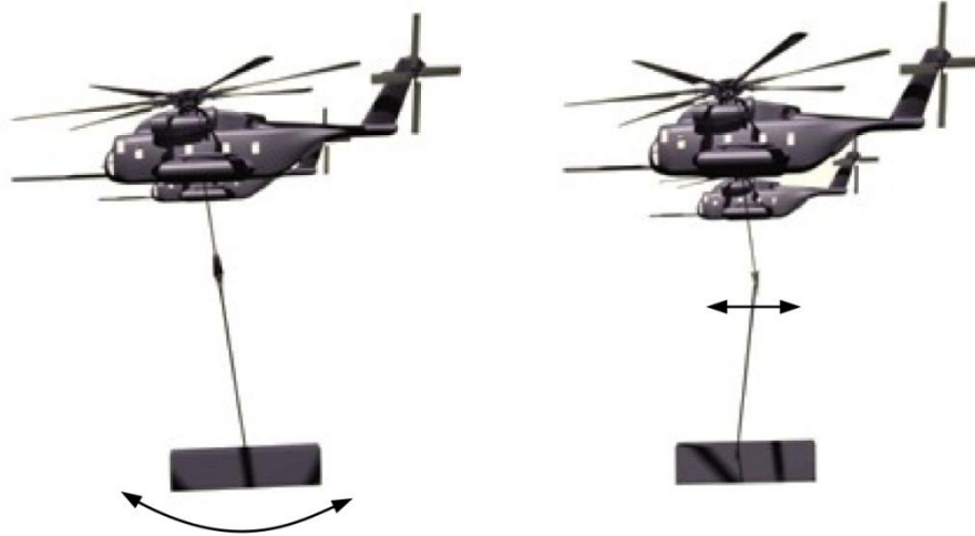
Figure 39: Double pendulum symmetric mode (left) and anti-symmetric mode (right)
